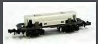
**K11-105** MOTORISIERTES CHASSIS 4-ACHS SPUR N
